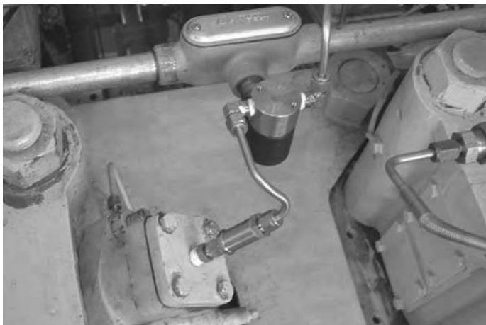
Pneumatic air distributor with pilot-actuated air-in-head valve
